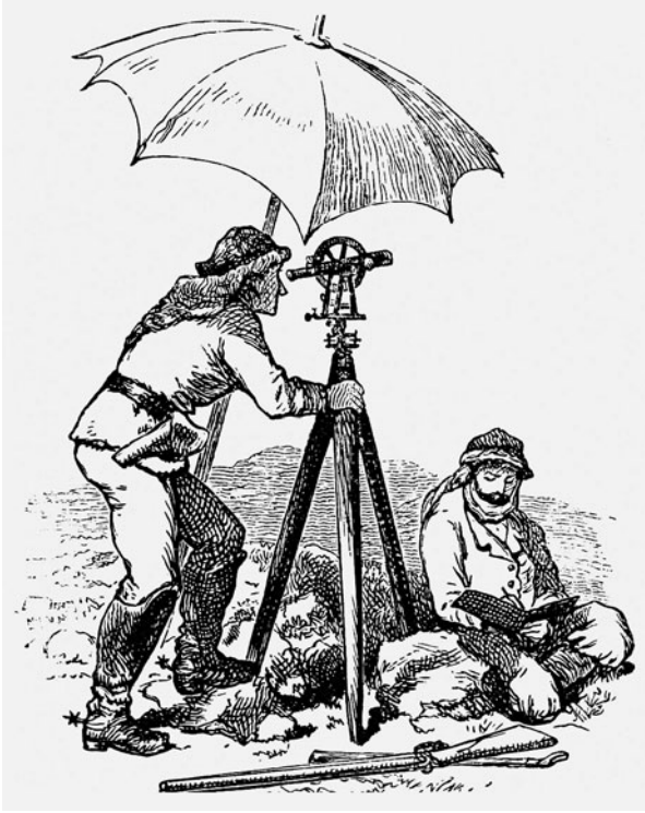
Figure 1.5 The first logo of the PEF; the image shows the methods used at that time to map: the theodolite and topographic triangulation. C. R. Conder, Tent Work in Palestine (London: Bentley, 1878), v. 1, frontispiece.
